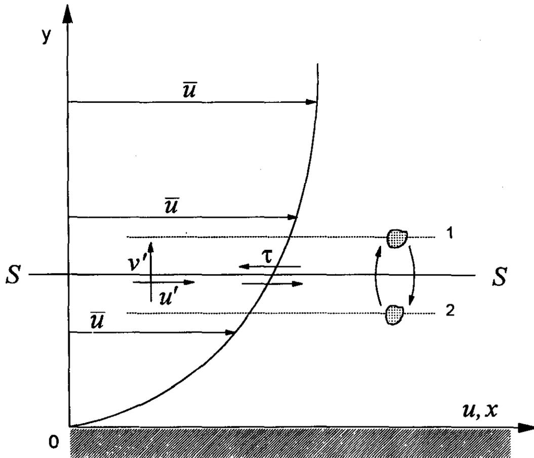
Figure 4.11 Turbulent momentum exchange in two dimensional flow.
