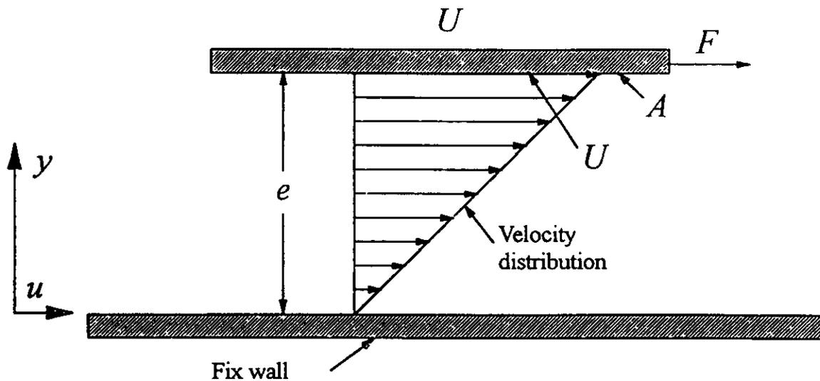
Figure 4.2 Shear stress applied to a fluid.
