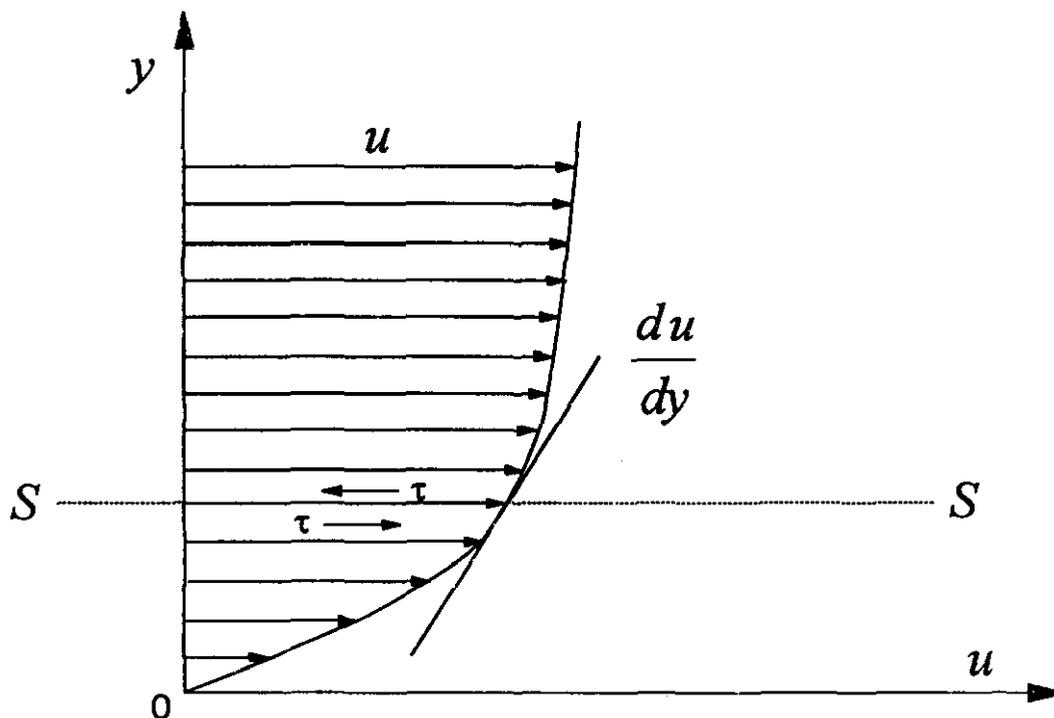
Figure 4.4 Velocity distribution next to a wall
