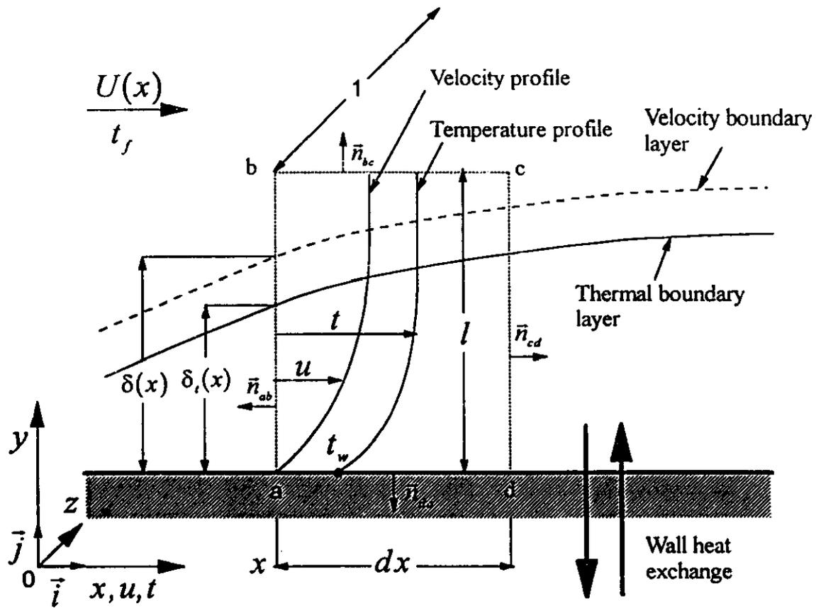
Figure 4.10 Control volume for integral conservation of energy
