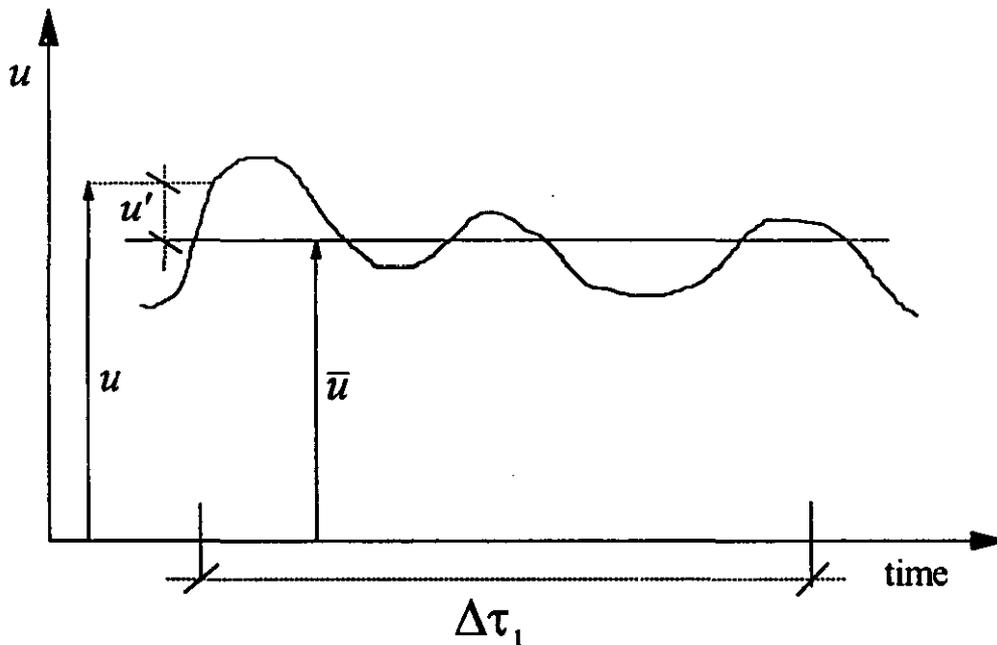
Figure 4.6 Turbulent velocity fluctuations about a time average.
