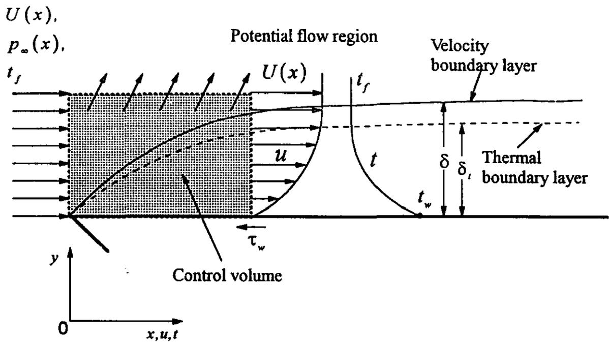
Figure 4.8 Velocity and thermal boundary layers in a laminar flow on a flat plate
